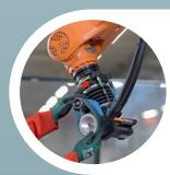
SUHNER Robotic Grinding: Automated surface treatment processes. Rough machining, grinding and polishing.
